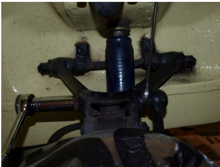
Tim's MGC Removing a tie rod from a just cleaned (after 2870 miles of mucky use in 2018) front wing October 2018
