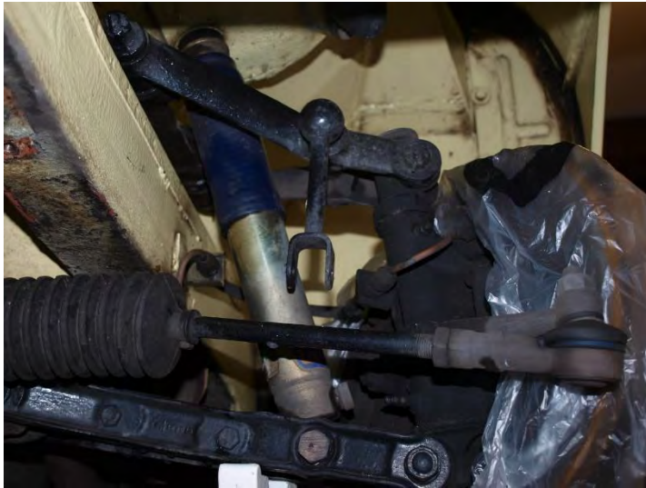
Replacing an anti-roll bar tie rod 2 weeks ago on our CGT. Not as clean as Jaimie Winfield's!!
